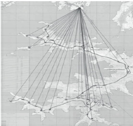
Fig. 3. Typical scheme for taking into account the principle of superposition of noise sources for calculation point No. 1
